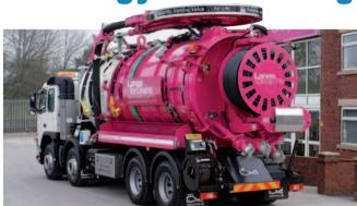
so, for example, has a tank made from 304 stainless steel, designed for non-hazardous waste. Also, its vacuum system is powered by a Mistral 402 exhauster-compressor and it caters for jetting, delivering 12gpm of water at 3,500psi.
